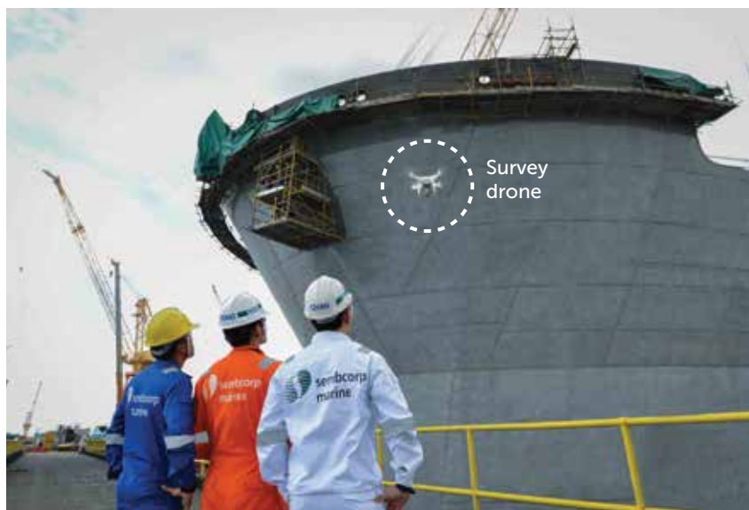
Drone technology has effectively mitigated the risks associated with conducting surveys in difficult locations
